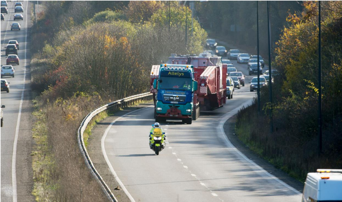
Image showing transportation of an offshore wind farm onshore substation transformer
